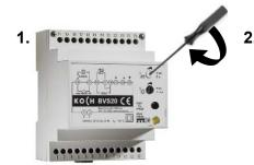
Set the length of time you would like the door to remain open (min. 0.8 s, max 8 s)
