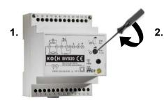
Set the length of time you would like the light to remain on (min. 0.8 s, max. 5 min).
